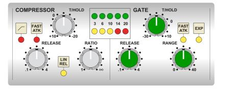
**THRESHOLD** – Variable hysteresis is incorporated in the threshold circuitry. For any given 'open' setting, the Expander/Gate will have a lower 'close' threshold. The hysteresis value is increased as the threshold is lowered. This is very useful in music recording as it allows instruments to decay below the open threshold before gating or expansion takes place.
